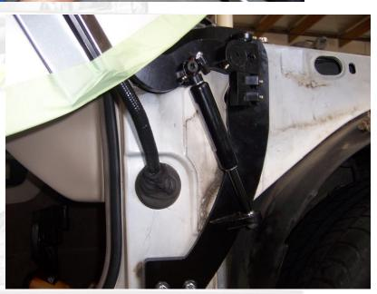
Note: cut the factory wire boot in half; half will be used for the body and the other half will be used for the door.
