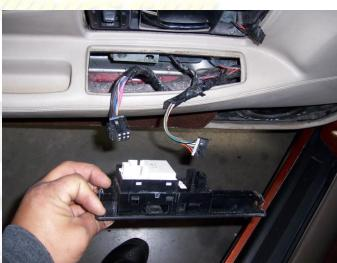
You will need more wire slack: Undue the clips holding the wires to the body, this will allow you pull the extra wire slack needed to raise the doors.
