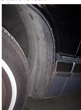
Remove all bolts or fasteners from the wheel well.
