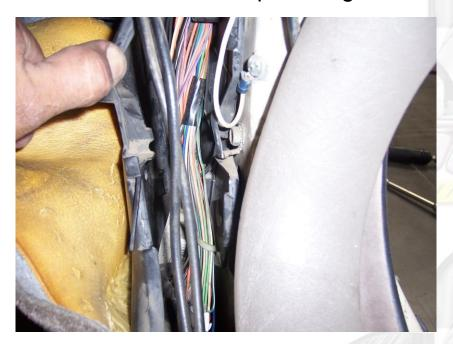
You will have to cut the factory wire boot in half; half will be used for the body and the other half will be used for the door. Use supplied wire loom to protect exposed wires.
