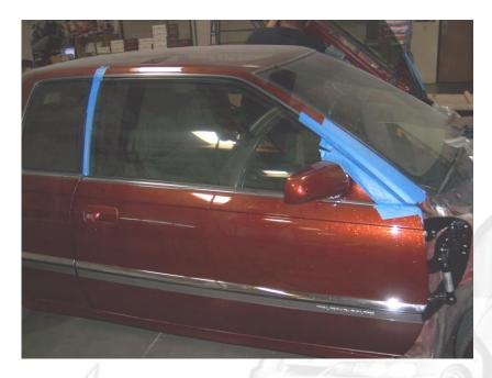
Make sure to mark how far the edge of the door is from the boy as shown in "PIC 1" top and "PIC 2" bottom.
