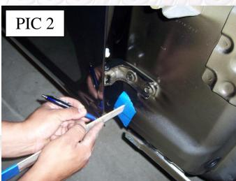
After making sure you have all the marks you need in case the door moves during installation, you can remove the factory door hinges. After installing the new VDI kit you should be able to raise the doors and start fine tuning you're your new VDI kit.
