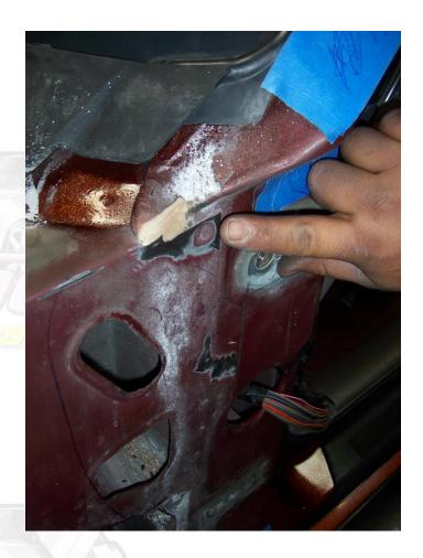
Place tape around the door and body of the vehicle as shown to help you locate the factory location. Then use 2" painters tape to
